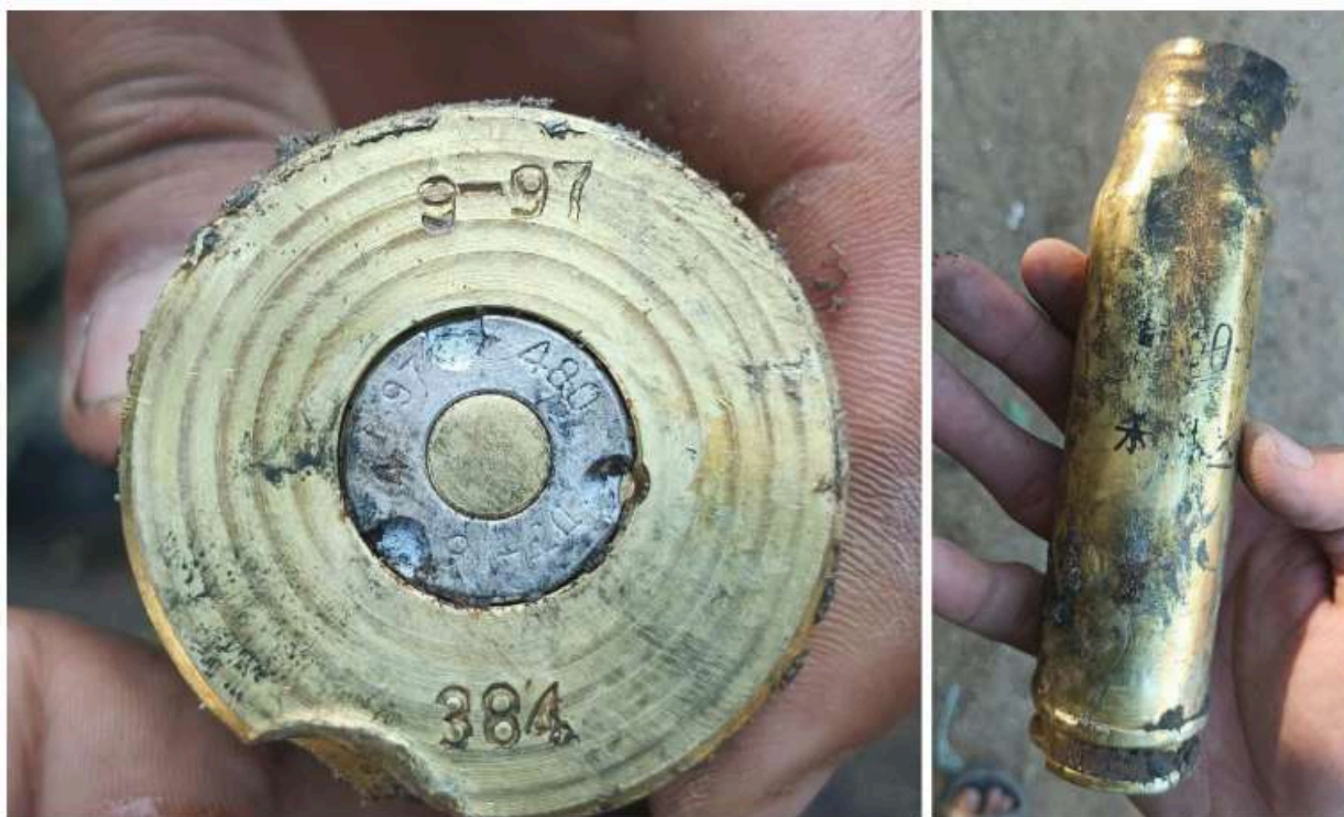
Figure 9: Myanmar Witness analysed equipment at the site of the crashed aircraft from UGC, identifying 1x 30mm round for aircraft cannon. Markings on the headstamp [Left] and shell casing [Right] suggest that this casing was manufactured or assembled in the People's Republic of China in 1997 (Source redacted due to privacy issues)
