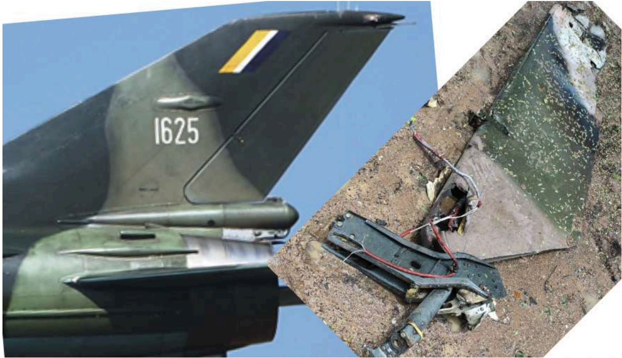
Figure 5: [Right] Myanmar Witness analysed components of the crashed aircraft from UGC, comparing it with the tail section [Left] of MAF F-7 tail number 1625 (sources: [Left] PLA and [Right] Airliners )
