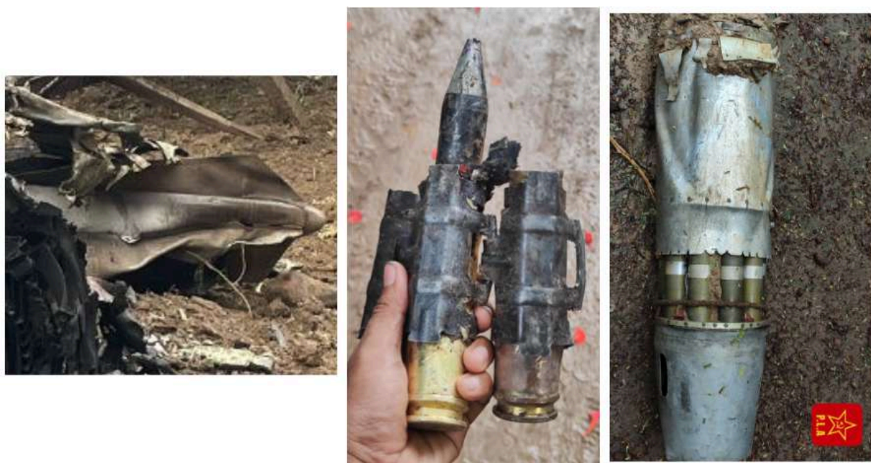
Figure 8: Myanmar Witness analysed components of the crashed aircraft from UGC, identifying [Left] 1x auxiliary external tank fuel, [Centre] 2x 30mm rounds for aircraft cannon, [Right] 1x pod for unguided rockets (sources: [Left] Mandalay Free Press , [Centre] PLA and [Right] PLA )
