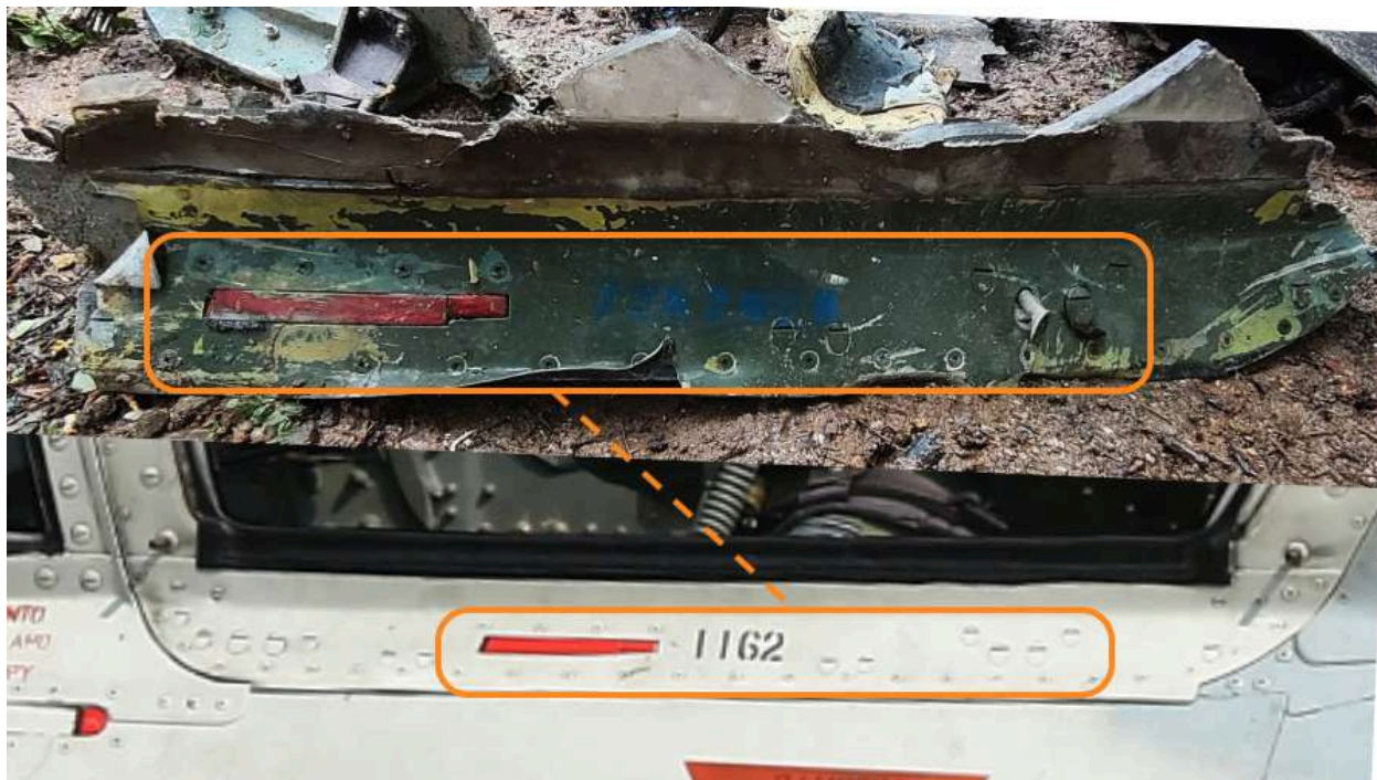
Figure 7: [Top] Myanmar Witness analysed components of the crashed aircraft from UGC, comparing it with the canopy [Bottom] of Bangladesh Air Force F-7 (sources: [Top] PLA and [Bottom] Wikimedia Commons )
